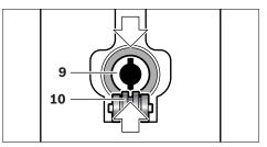
**Note:** If the grooves of the saw blade holder are not in the position shown in the figure, then the saw blade **12** cannot be inserted into the stroke rod **9**. Briefly press the SDS clamping lever **8** toward the side and release it again.
